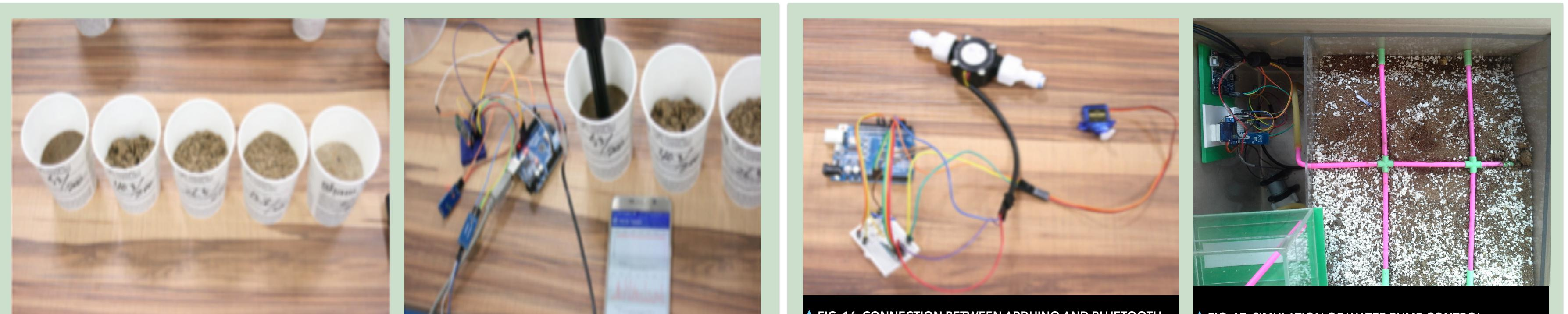
FIG. 11(A). SOIL MOISTURE LEVEL: 100%, 75%, 50%, 25%, 0%
