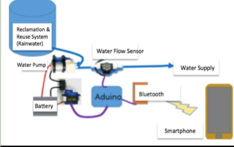
FIG. 15. CONNECTION THROUGHOUT WATER SUPPLY CONTROL
