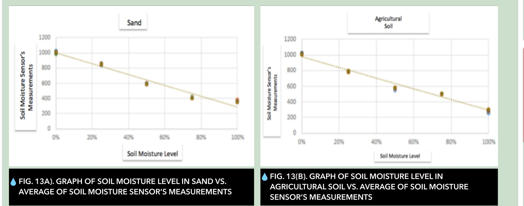
Both experiments with sand and agricultural soil portrayed inverse linear relationship between soil moisture sensor measurement and soil moisture level. The results confirmed that low moisture corresponded to high resistance and high moisture corresponded to low
